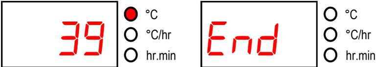
When the kiln has cooled to less than 40°C the display alternates every 5 seconds between the kiln temperature and *End*
