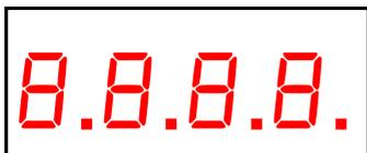
When turned on the ST312B performs a display test by briefly illuminating all of the display digits and all of the front panel lamps.
