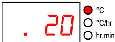
If the left-hand decimal point is on then the keyboard is locked & the ST312B will not respond to the START/STOP key. Press the  $\uparrow$  &  $\downarrow$  keys together & hold down for 5 seconds to unlock.
