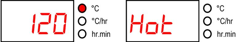
While the kiln temperature is above 40°C the display alternates every 5 seconds between the kiln temperature and *Hot*
