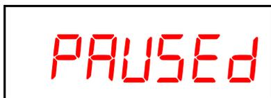
As a warning during pause a double beep is sounded every 10 seconds, the display scrolls *PAUSED* for 5 seconds then shows the kiln temperature for 5 seconds.
