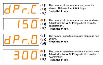
The ST215C will now reset and the new damper control temperatures will be stored.
