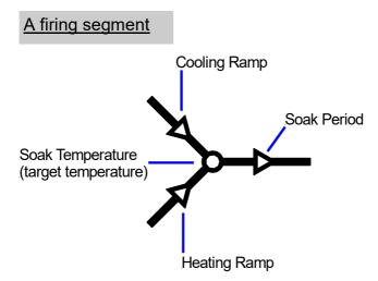
An ST215C firing segment comprises a ramp followed by a soak period. Two segments can be used for simple firing (biscuit firing for example) or several segments can be used per program for complex firing (crystal glazing or glass-making for example).
