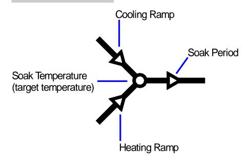
An ST535 firing segment comprises a ramp followed by a soak period. Two segments can be used for simple firing (biscuit firing for example) or several segments can be used per program for complex firing (crystal glazing or glass-making for example).
