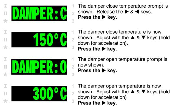
The instrument will now reset and the new damper control temperatures will be stored.
