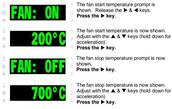
The instrument will now reset and the new fan control temperatures will be stored.
