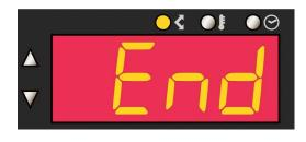
Explanation: the full range of displayed values for ramp rate are: End, 1...999°/hr, FULL. To mark the end of a program select a ramp rate of "End" by holding down the DOWN key until End is displayed. To add an extra segment press the UP key until your desired ramp rate is shown. If you want to heat at full power hold down the UP key until FULL is displayed.
