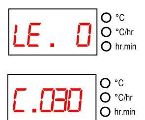
Lock-up on error status is now displayed. This can be altered with the **↑** & **↓** keys. LE. I indicates that lock-up on error is enabled. LE. [] indicates that lock-up on error is disabled. Press the START/STOP key.
