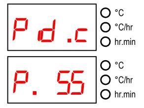
If the START/STOP key is pressed when this menu is shown then the menu for reviewing or changing P (the proportional band) is shown:-
